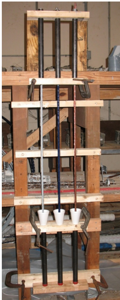
Figure 2-2: Setup used to cast the ends onto the strands; setup has three different strand types that have already been cast.
