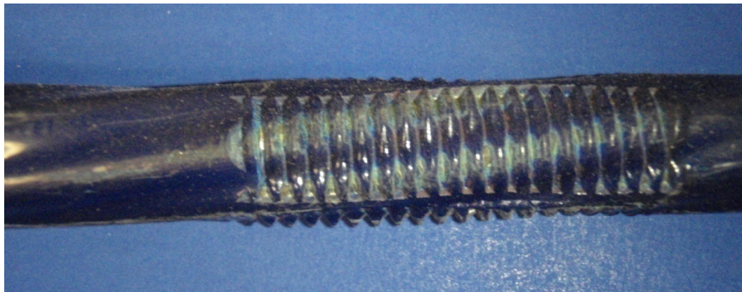
Figure 4-11: Flow filled epoxy coated strand showing damage done by chuck
