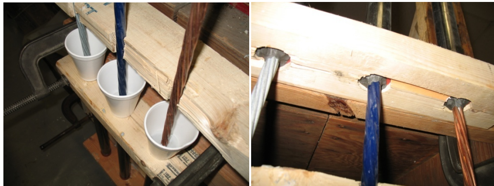
Figure 2-5: Left: close up of the Styrofoam cups at the top of the bottom piping with the strands inserted ready for casting; Right: close up of the bottom of the top piping showing the epoxy putty which has hardened and is ready for casting.
