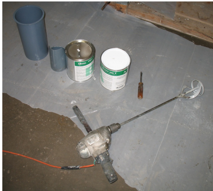
Figure 2-6: 2 part epoxy used to cast ends and mixing apparatus including the high shear blade and variable speed drill.
