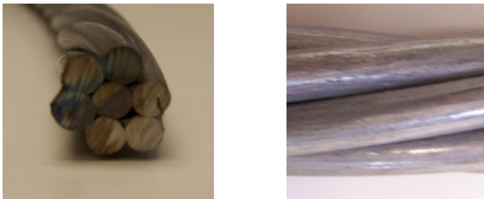
Figure 1-3: 0.6 in. stainless steel strand 1
