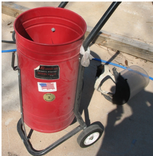
Figure 2-1: Abrasive Blaster used to sand blast the ends of the strands.
