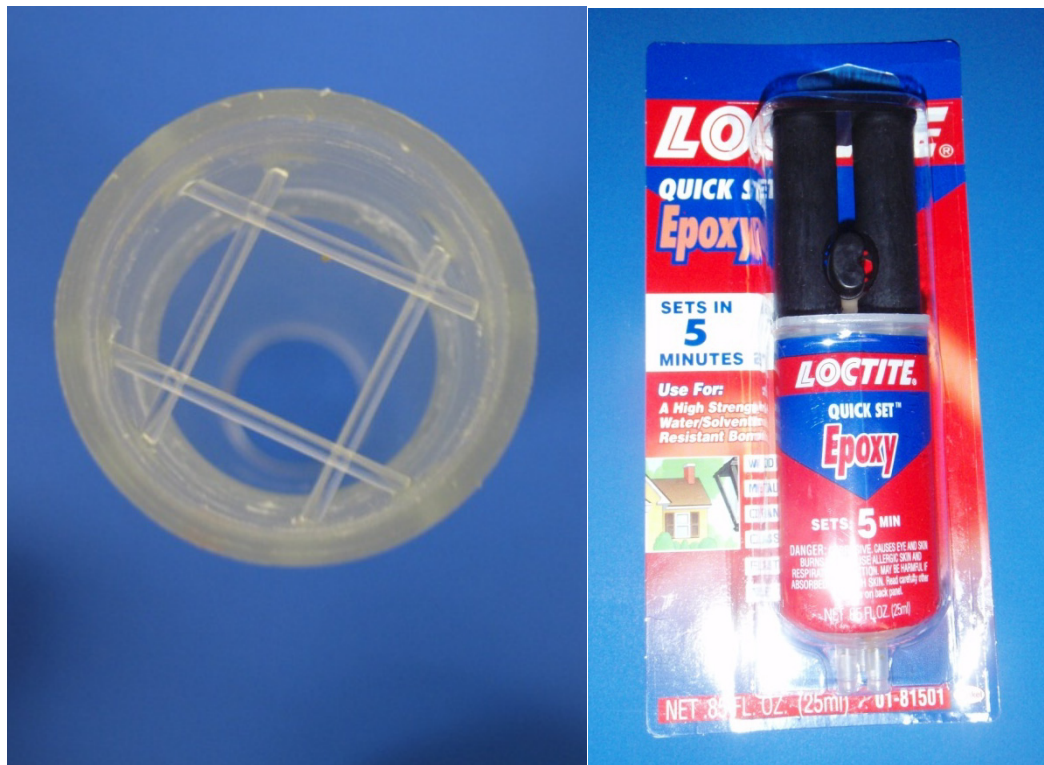
Figure 4-9: Specimen part showing acrylic rods and epoxy
