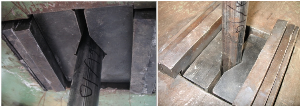
Figure 2-9: Step 1: Ends secured in the V-grips of the test machine.
