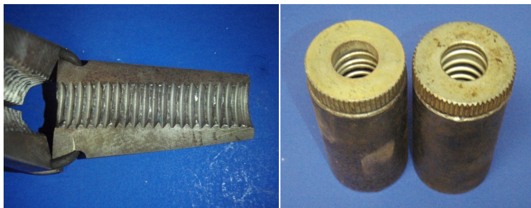
Figure 4-12: Chucks used to damage epoxy coating
