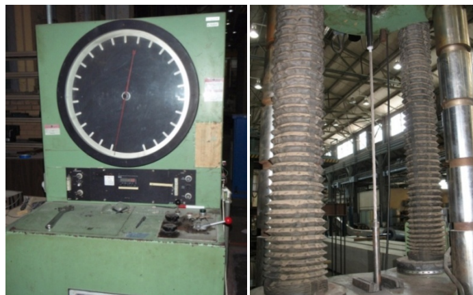
Figure 2-7: SATEC Systems Inc. 600 kip testing machine with strand specimen in place.
