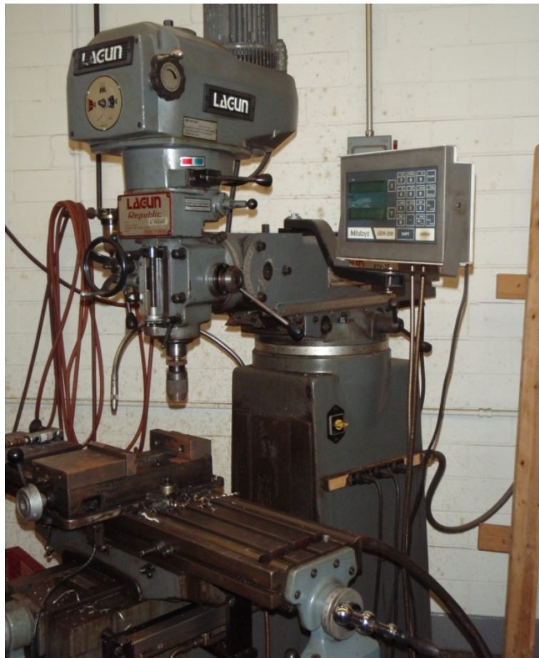
Figure 4-7: Lagun Republic milling machine
